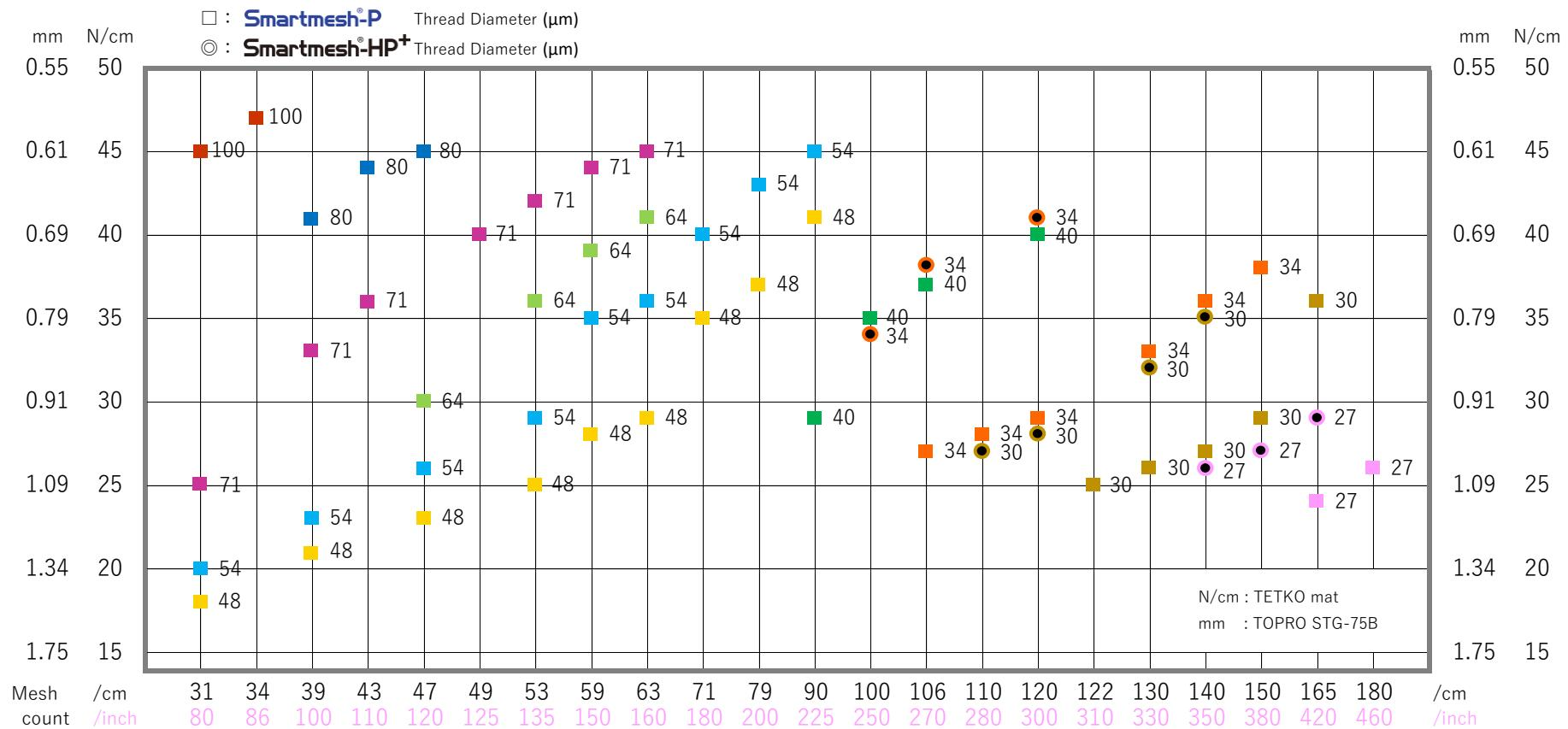
The values shown in the above figure are the recommended maximum tension values when a screen mesh is stretched with a mechanical screen mesh stretching device (Size: 1,000 mm x 1,200 mm). Tension values are affected by various factors, such as the type and drive system of the screen mesh stretching device, as well as the mechanical, pneumatic, hydraulic, and screen mesh stretching conditions.
